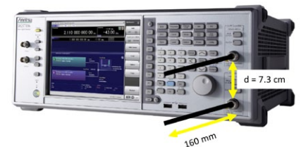
Figure 2: beam-forming antenna set-up using the Anritsu MG3710A signal generator's two RF ports.
